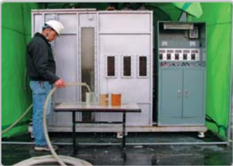
Installation and operation of the system at S Chemical for treating pigment waste water.
